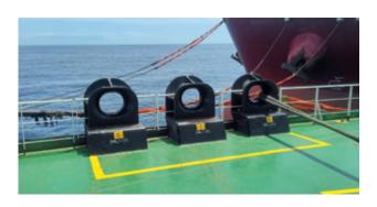
A step-change within this element of the operation, the mooring fuse ensures that potential over-tension is identified and managed before it causes damage, without compromising the integrity of the ship mooring system.
