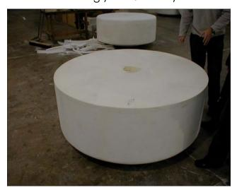
used only as secondary fenders. These fenders usually consist of a closed-cell polyethylene foam material which is wrapped on to a mandrel to give a finished diameter.
