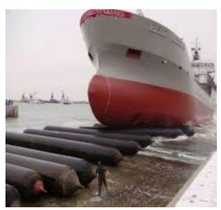
Airbags work well in a ship launching situation. When deployed, there are usually many units in place and the failure of one is not likely to be a major problem.
